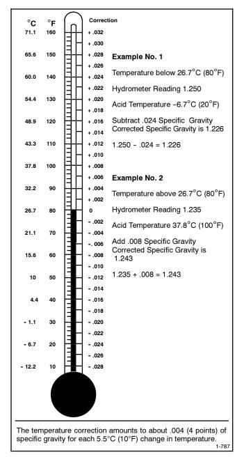
Figure 3-20 Specific Gravity Temperature Correction
